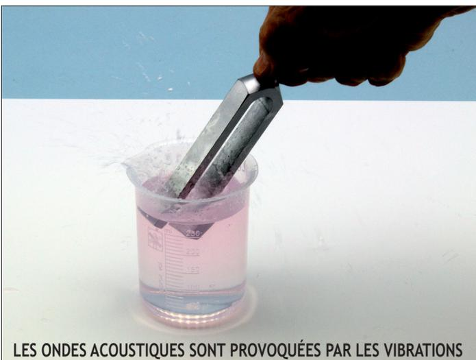
LES ONDES ACOUSTIQUES SONT PROVOQUÉES PAR LES VIBRATIONS
